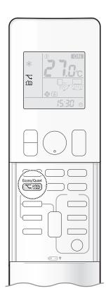
ECONO operation enables efficient operation by limiting the maximum power consumption. This function is useful to prevent the circuit breaker from tripping when the unit operates alongside other appliances on the same circuit.
