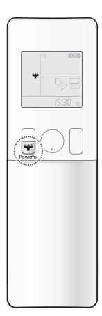
POWERFUL operation quickly maximises the cooling effect in any operation mode. In this mode, the air conditioner operates at maximum capacity.
