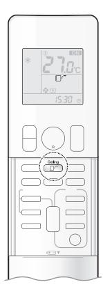
The flow of air will be in the upward direction while in COOL/FAN/DRY operation, which will provide a comfortable wind that will not come in direct contact with people.
