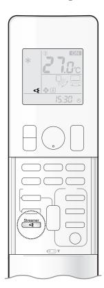
The streamer generates a high-speed electron stream with a high oxidizing power, reducing bad odours and viruses. Together with the air quality filter (enzyme blue with PM2.5) and the air filters, this function cleans the air in the room.
