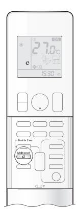
The inside of the air conditioner is dried to reduce the occurrence of mold and odour.
